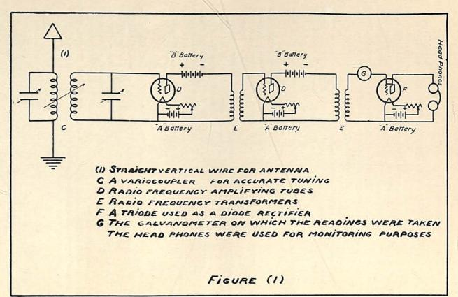
Galvanometer readings proportional to energy received.
