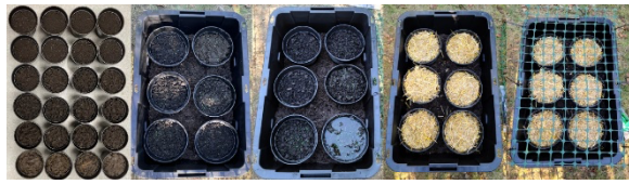
Figure 1. Progression of study preparation (from left to right: topsoil and sludge mixing, seeding, watering, straw layer, and final setup).
