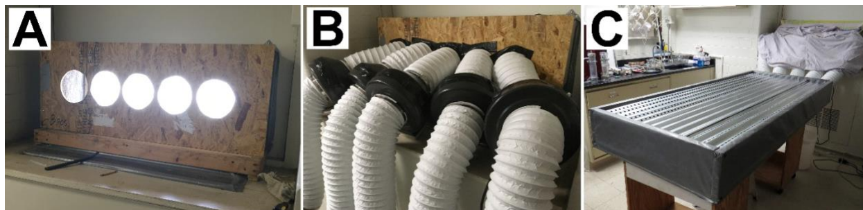
Figure 1. The downdraft table and local exhaust ventilation system. (A) An air conditioning unit was removed from its casing and a piece of oriented strand board with five holes to accommodate 6-inch flexible ducting (diameter ~15 cm) was affixed to the casing. (B) Flexible ducting was affixed to 6-inch inline duct fans which were wrapped with duct tape to prevent vapors from exiting seams in the fan casing. (C) The downdraft table was placed atop two carts and joined to the flexible ducting. Ducting, fans, and the retrofitted window casing were covered with towels and blankets as an added precaution to ensure that vapors would not spread into the room from any potential leaks in the system.
