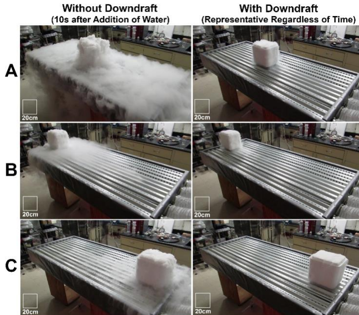
Figure 3: A side-by-side demonstration of the capacity of a simple downdraft table paired with a simple local exhaust ventilation system to exhaust water vapor (generated by pouring warm water into a container of frozen carbon dioxide). Images were captured from video 10 seconds after the addition of the water in the absence of downdraft (left column). In the absence of downdraft, water vapor rapidly escaped the perimeter of the downdraft table. In the presence of downdraft (right column), the downdraft table removed water vapor consistently and prevented water vapor from moving along the tabletop surface. Accordingly, the downdraft prevented the water vapor from escaping the perimeter of the table. (A) Dry-ice container located in the center of the table. (B) Dry-ice container located away from the exhaust manifold. (C) Dry-ice container located near the exhaust manifold. NOTE: This Figure corresponds to Video 1 .
