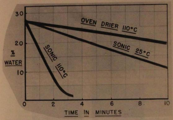
FIGURE 15. Drying of powdered coal layer 0.6 cm in thickness in drying oven with and without ultrasound.
