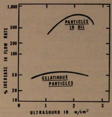
FIGURE 12. Curves showing increased filtration rate produced by adding ultrasound into system. Top curve is for 7.5% slurry containing 1-40  $\mu$ m particles in 30W motor oil. Bottom curve is filtration of neutralized mine water drainage.
