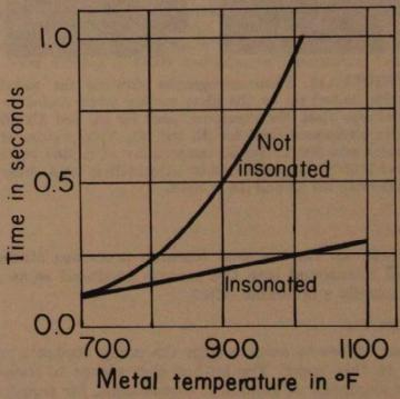
FIGURE 16. Adherence curves showing the influence of ultrasonics on the retention time of molten glass beads on the heated cast metal surface.
