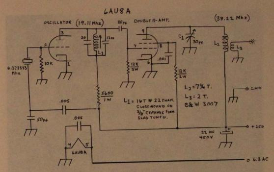
FIGURE 7. Circuit diagram for the acousto-modulator driver.
