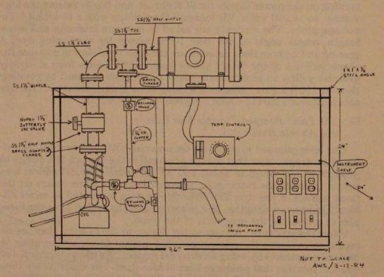
FIGURE 13. Chamber and vacuum system for laser spectroscopy.
