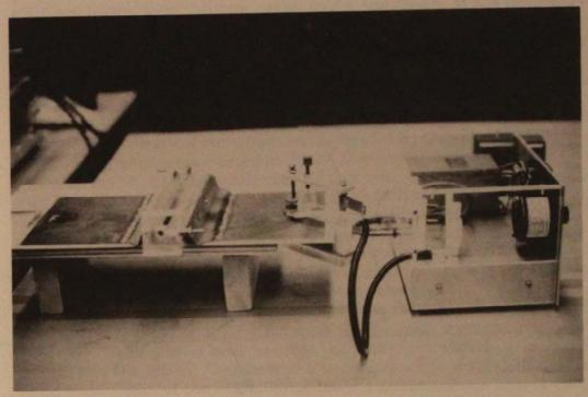
FIGURE 10. The nitrogen laser, Blumlein design.
