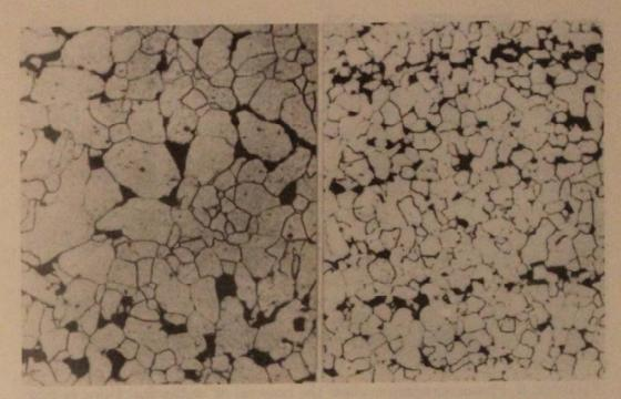
FIGURE 4. Photomicrographs showing the influence of insonating low carbon steel upon the grain size produced during polymorphic transformation. White grains are ferrite, black grains are pearlite. Magnification is 100X. Right sample ultrasonically treated.
