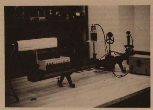
FIGURE 3. Experimental arrangement for the Kerr Effect.
