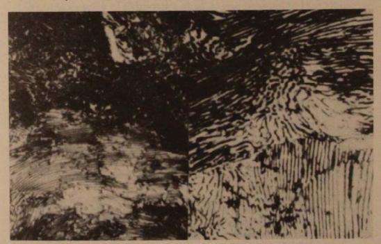
FIGURE 5. Photomicrographs showing the influence of insonating high carbon steel upon the lamellar layer thickness of the ferric and iron carbide produced during polymorphic transformation. Magnification is 1000X. Right sample ultrasonically treated.
