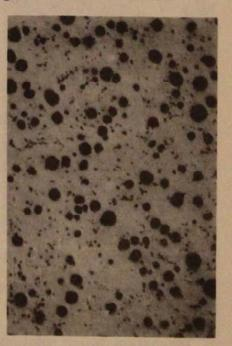
FIGURE 3. Photomicrographs (50X) showing the influence of ultrasound on the size and distribution of the graphite nodulars formed during solidification of the iron.
