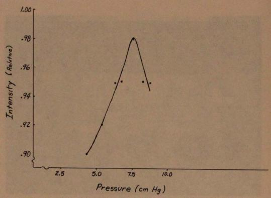
FIGURE 11. Intensity versus pressure for the nitrogen laser (by J. Puddington, Class of 1983).
