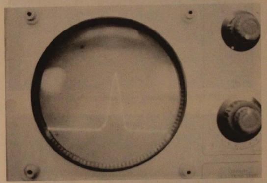
FIGURE 2. Profile of the He-Ne laser beam measured with photodiode array.
