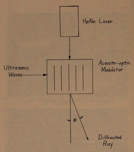
FIGURE 6. Schematic of the Acousto-Optic Effect experiment.
