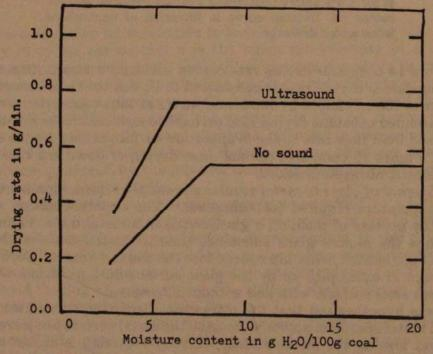
FIGURE 14. Typical drying rate curves showing the effect of airborne ultrasound being introduced above the evaporation surface.
