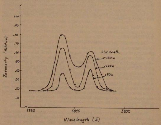
FIGURE 1. Measurement of sodium doublet with monochromator (by B. Douthitt, Class of 1982).
