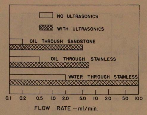
FIGURE 13. Bar graphs showing increased flow rates produced when adding ultrasound into system. Sandstone had 20% porosity with flow channels of 10-50  $\mu$ m in size, stainless steel filter had 42% porosity with flow channels of 20-180  $\mu$ m in size.
