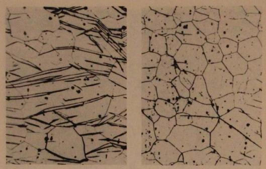
FIGURE 6. Photomicrographs show the removal of mechanical twins in magnesium by insonation of specimen which were mechanically deformed 12%. Both samples were heated to 500°C for 30 minutes. Magnification is 100X.
