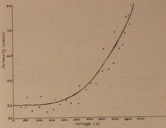
FIGURE 5. Intensity versus voltage for the Kerr Effect (by B. Longacre, Class of 1983).
