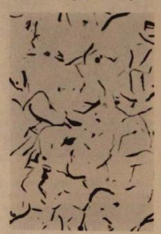
FIGURE 2. Photomicrographs (25X) showing the influence of ultrasound on the graphite size formation and distribution during solidification of the iron.
