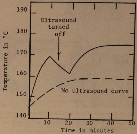
FIGURE 9. Unsteady state temperature curves showing the effect of introducing ultrasound in a magnesium bar. The lower dashed curve is for no sound added. Both curves continue to a steady state condition.
