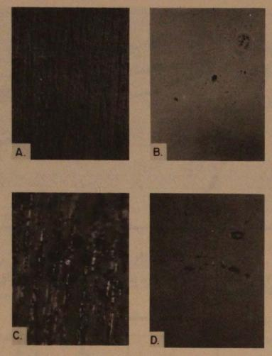
FIGURE 17. Photomicrographs showing the metal oxide picked up by the glass surface when cooled on stainless steel. No ultrasound used for (A) and (C). 20 kHz ultrasound used for (B) and (D). Temperature of metal was 500°C. Initial temperature of molten glass was 1100°C. Magnification for (A) and (B) is 100X. Magnification for (C) and (D) is 500X.
