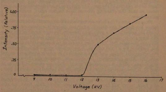
FIGURE 12. Intensity versus voltage for the nitrogen laser (by J. Puddington, Class of 1983).
