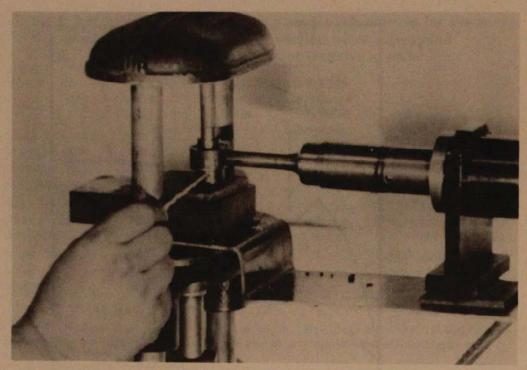
FIGURE 11. Photograph showing extrusion of ultrasonically-heated polymer powders. Vertical plunger compresses powder in cylinder which has small extrusion hole near bottom on side. 20 kHz vibrations are introduced into wall of cylinder from the ultrasonic horn.
