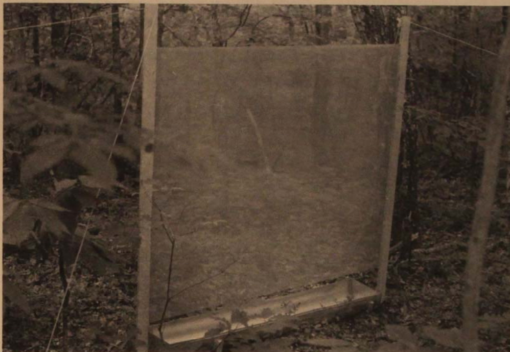
FIGURE 1. Large-area flight-intercept or "window" trap.
